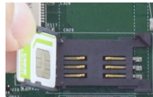
Insert SIM card with pins facing up
