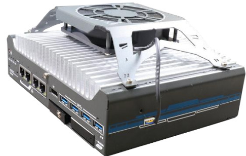
Insert the 4-pin plug properly
