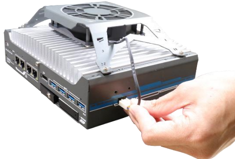
Locate 4-pin power plug location
